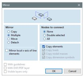
Select Multiple Mirror type and set None for Nodes to connect.
