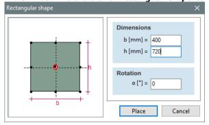
Enter **720** for height (**h[mm]**=) and click on **Place** button. (The **b** size of the rectangle shape is equal to the default value, so it does not have to be overwritten now.) Click anywhere in the workspace to place the cross-section. The following result can be seen:
