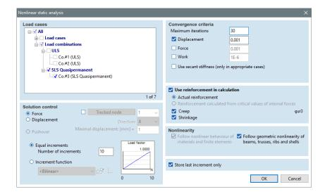
The only purpose of the nonlinear analysis is to study the deformation of the structure, so check **Co.#3** (**SLS Quasipermanent**) load combination in **Load cases** list. Check **Use reinforcement in calculation**, and considering **Creep** and **Shrinkage**. Set the other parameters according to the above window. Start analysis by pressing **OK** button, the following shows up:
