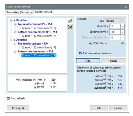
As we can see, the rebar position is calculated automatically taking into account concrete cover, the position of each reinforcement layers and the diameters of the applied rebars.
