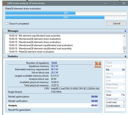
The **Estimated Memory Requirement** shows the necessary amount of memory to run the analysis. If this value is higher than the available physical memory, then **AxisVM** uses the hard disk to swap memory blocks during the calculation. If the system of equations fits into the physical memory the calculation is considerably faster.
