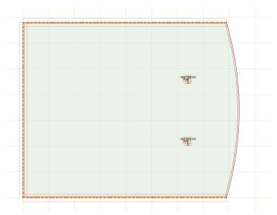
Change result component to *Rz [kN/m]* in group *Line support internal forces*. Activate *Result display parameters* window and check *Write values to Lines* function to see the result values.
