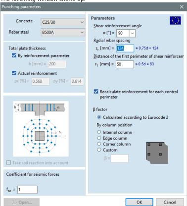
The material types (for concrete or rebar) are set automatically applying the parameters set before. Programs applies the current design code and national specifications. Set the parameters shown above and click on **OK** to close the window. We get the following results:
