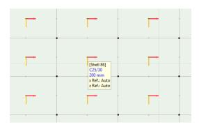
The red line shows the x axis of the local coordinate system, the yellow one the y axis and the green one the z axis.
