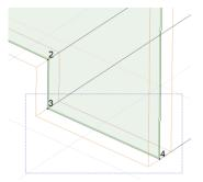
All the elements within the rectangle will be selected (**node 3**, **4** and the line between them). To move the line, move the cursor over the selected line, press and hold the left mouse button and drag the cursor down.
