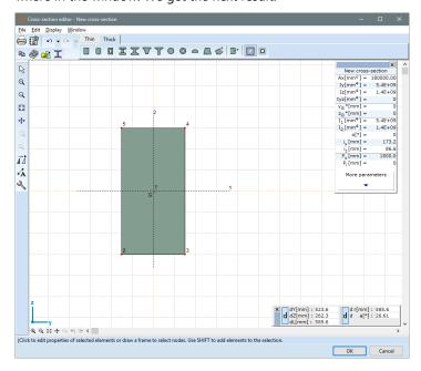
The 1st and 2nd principal direction of the cross section indicated by the crossing dashed lines on the cross-section, marked with numbers 1 and 2. The centre of gravity is marked with G. The other cross-section parameters are displayed within the property window. Click *More* parameters if you want to see all parameters calculated automatically by a finite element analysis of the shape.
