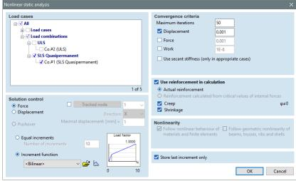
At **Load cases** select **Co.#1 (SLS)** load combination and check **Actual reinforcement** to use in calculation, and let us consider the effect of **Creep** and **Shrinkage**. By clicking on **OK**, then the analysis starts:
