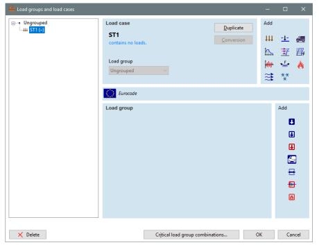
In the window that appears, click on the name **ST1** in the top left corner and rename it to **SELF-WEIGHT**. (**ST1** is an automatically generated load case, which should be renamed in our example.)
