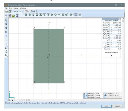
Notes: **Stress calculation points** are automatically placed at the corners and at the centre (please see numbering 1..5). Stress is calculated only in these predefined points. These points can be modified or cleared or more points can be added. In our analysis there is no need for these points because the longitudinal reinforcement is calculated directly from internal forces.
