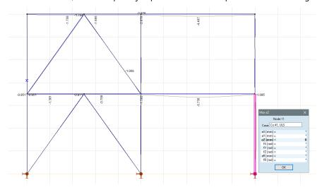
Select **Beam internal forces** – **Nx [kN]** component from the drop-down list among result components.
