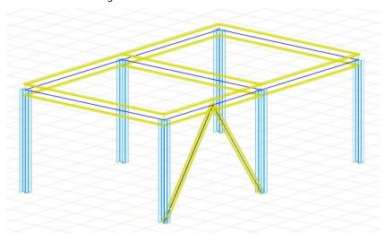
Press *Esc* to close polyline function, then repeat previous steps to specify the bracing elements on the other side of the structure.
