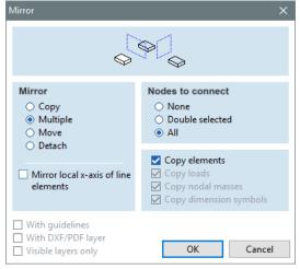
Select *Multiple* mirror type and *All* for *Nodes to connect*, then confirm with *OK*.
