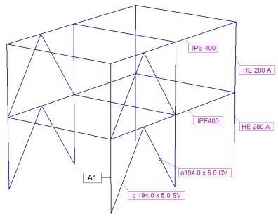
Consider IPE 400 rolled steel cross-section for horizontal beam elements and HEA 280 for columns. The cross-section of bracing elements is O194.0  $\times$  5.0 SV. Use material S235 and apply Eurocode standard for the design.
