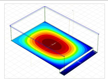
R. C. design To analyse the required reinforcement of the reservoir, change tab to R. C. design:
