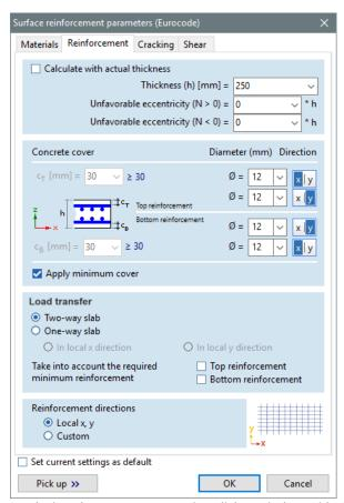
By closing the parameters setting dialog window with **OK**, the results of calculated bottom reinforcement in local **x** direction - **axb** [mm²/m] can be seen on the screen. Change **Display mode** to **Isosurfaces 2D**.
