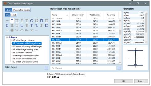
Roll down in the list of *Cross-section tables* by using vertical sliding bar (or roll mouse wheel) and select *HE European wide flange beams*, and click on *HEA 280 A*. Finish with *OK*.
