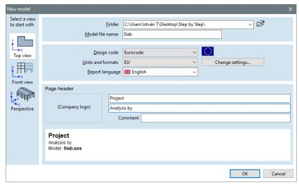
Starting workplane also can be set on the left in this window. Change workplane to **X-Y Top view**. Our slab will be parallel to this plane, and the gravity load acts in **-Z** direction. This setting can also be done using **Choosing view** icon on the editing interface.
