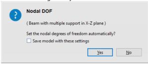
In our model the beam is not fixed in **Y** direction, on the other hand it is free to rotate around **X** direction. Please note: the software only filters out the basic faults in the data input, but cannnot find every fault beforehand that can cause problem in the stiffness matrix.
