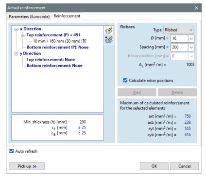
Click on the field of given reinforcement at **Top reinforcement** in **x Direction**, after click on **Top reinforcement** in **y Direction**. Finally, add the specified reinforcement to the last selected layer:
