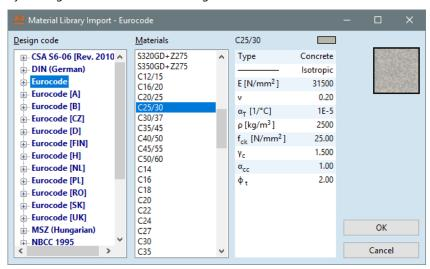
Roll down in the list of *Materials* by using the vertical sliding bar (or simply roll down the mouse wheel) and select *C25/30*, then click on *OK* to close the window.
