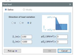
To define water level **30 mm** under the top edge of the reservoir change **Z1** [m] = **3.000** to **2.7**, and set the bottom pressure value  $p(Z_2)$  [kN/m²] to -35 (pressure is in the negative local z direction) and click **OK**. The following will be displayed:
