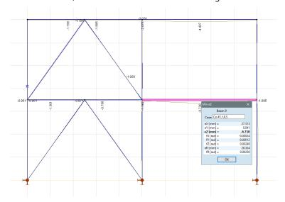
After click on **OK**, the result panel jumps to the maximum positive value showing its location.
