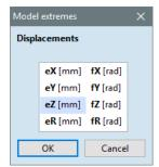
Select one of the deformation components. Confirm with **OK**, then the program shows maximum negative value and its location as well:
