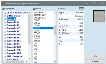
Roll down in the list of *Materials* by using vertical sliding bar (or roll mouse wheel) and click on *C25/30*, then click on *OK*.
