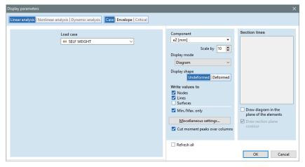
Select **SELF WEIGHT** load case and result component **Displacement**, **ez [mm]**. Change **Display mode** to **Diagram**. If we leave **Display shape** on **Undeformed** the results are drawn to **undeformed** model. Check **Lines** and **Nodes** boxes at **Write Values to** setting.
