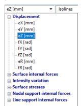
Select **Surface internal forces** – **mx [kNm/m]** then **mx** moments will be displayed in **Isolines** mode. The **mx** specific moment represents the moment that rotates around local **y** axis. With same method, select and see the following result components: **my**, **mxy**.
