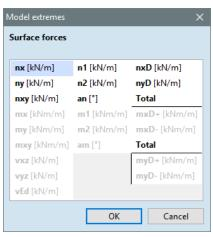
Select one of the *Surface force* components. Confirm with *OK*, and the program shows the negative maximum value and its location as well.
