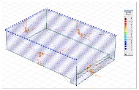
All domains are hatched in blue what denotes that there are no cracks on outer face of domains. Check crack widths on the inner face of the reservoir!
