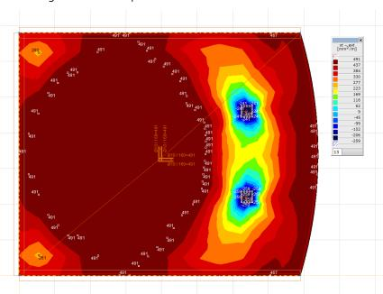
Around the nodal supports negative values can be seen indicating the areas where additional reinforcement must be applied.
