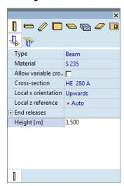
Note: in the window several parameters can be set which are not mentioned here. *End releases* can also be specified or the local coordinate system of the element can be modified. In our example, we use default setting for these. (The end releases of an element are fixed by default settings.)
