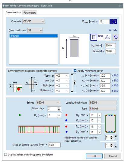
Specify rectangular shape for the rib on *Cross-section* tab, and select *S3 structural class*.
