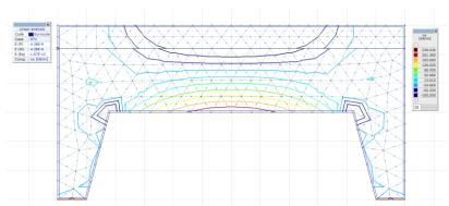
View internal forces of the supports. Select *Rz* component between *Line support internal forces* in the *Result component* combo box.
