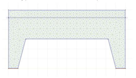
Finish the selection with **OK** and type in  $p_y$  [kN/m] to 50:
