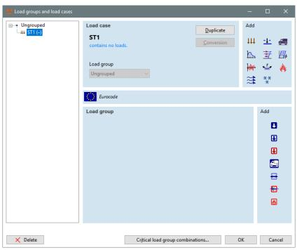
The software automatically generates load case **ST1** which can be seen in the list on the left. Click on the name of **ST1** and rename it to **SELF WEIGHT**. Then click on OK button to go back to model space. The last edited load case (named **SELF WEIGHT**) will be the active case, this can be checked on **Status** panel in the top left corner of the screen.
