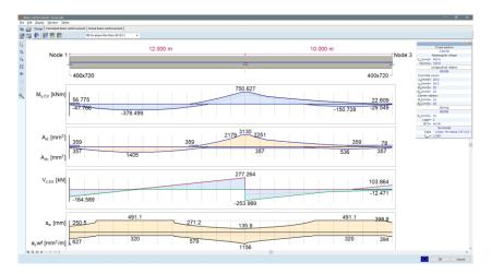
After clicking on *Calculated beam reinforcement* tab, the following diagrams can be displayed: Envelope of reinforcement (*As*), cracking (*wk*), moment resistance (*MyRd*), maximum shear force (*VzRd*), relative deflection (*ez,rel*), absolute deflection (*ez,abs*). To display other types of results and diagram set the *Display parameters*.
