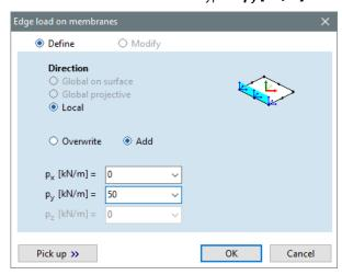
Press **OK** and the load is applied. The following result is displayed:
