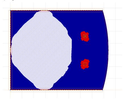
It can be seen that there is no need for upper reinforcement in the middle, hatched area of the slab. In the blue areas **Ø10/160 mm** base reinforcement is needed, and in the vicinity of the columns extra reinforcement must be applied (**Ø10/160 mm**+ **Ø10/160 mm**).
