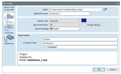
(Starting workplane (**X-Z** plane/front view) can also be set in this window if selected from the list in the left side.)
