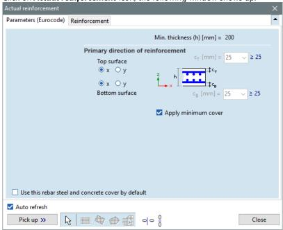
Firstly, the base reinforcement (**Ø10/160 mm**) will be specified in each direction, the extra reinforcement will be added to actual reinforcement later.
