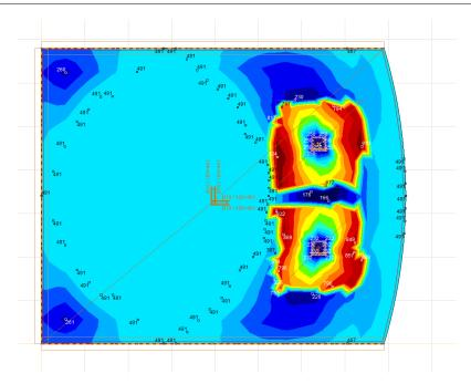
There is not any negative **xt-axt** value, so the actual reinforcement is sufficient at top in **x** direction. Now select **yt-ayt** result component. The negative values show that we also need additional reinforcement at top in **y** direction.
