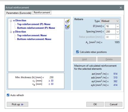
Set reinforcement rebar on right hand side and assign it to each four reinforcement layers on left hand side.
