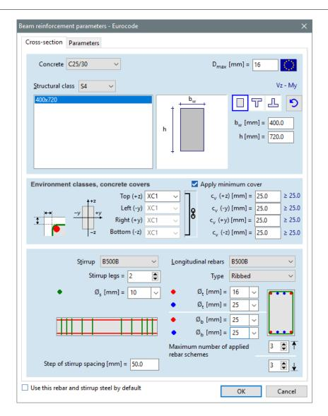
On *Cross-section* tab the cross-section of the beam can be modified if it necessary, but please note that the internal forces will be recalculated only if a new static analysis is done. So, this option should be used only in justified cases.
