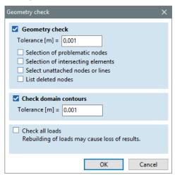
Switch off the option of **Select unattached nodes or lines**, then close the window with **OK**.
