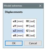
Select **ez** and click on **OK**. The result panel shows the highest negative deformation and its position, after clicking on **OK** the highest positive deformation is shown. Click again on **OK** to close.
