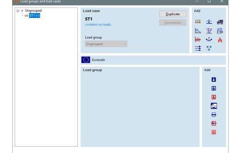
In the window that appears, click on the name **ST1** in the top left corner and rename it to **LIVE 1**. (**ST1** is an automatically generated load case, which should be renamed in our example.) Close window with **OK**, then the previously edited load case (**LIVE LOAD 1**) is active. The actual load case is indicated on **Info palette**, shown below:
