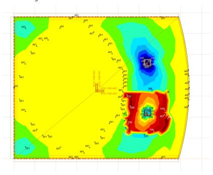
The results of **xt-axt** component around the bottom lower nodal support are positive, so the actual reinforcement is sufficient with the additional reinforcement.
