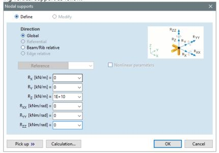
If the support conditions are set correctly, the given non-zero components of the support are indicated by brown symbol on the screen.
