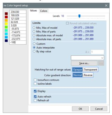
Press *Enter* to finish data entry and switch on *Auto interpolate*. This option will recalculate the inner boundary values depending on the number of boundary levels.
