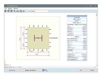
The required dimensions and reinforcement are shown in plain view and in *Info window*. The view can be rotated as usual or a perspective view can be requested, if necessary (see *Display* menu). By clicking on *Settings* icon, the desired display parameters can be set.
