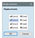
Select one of the deformation components: **eY [mm]**. Click on **OK** to show maximum negative value and its location.
