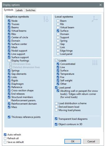
In Local systems group, check Surface checkbox and close window with OK.
