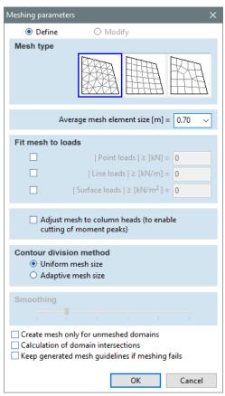
Type in **0.7 [m]** for the **Average mesh element size**. After closing the dialog with **OK**, the automatic mesh generation starts. The progress of **Mesh generation** is shown in the window:
