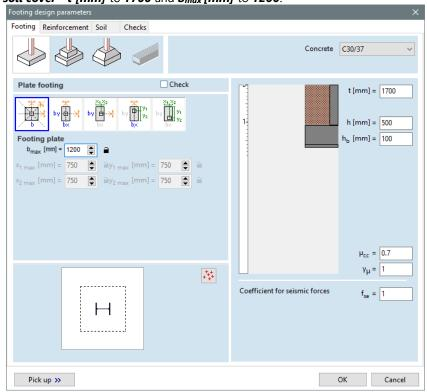
On reinforcement tab check *Calculate reinforcement* and *Punching reinforcement* function, and set reinforcement parameters as shown below:
