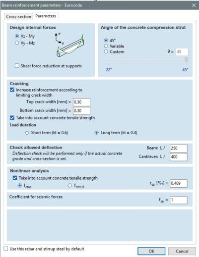
Checking **Shear force reduction at supports** allows the application of shear force reduction methods according to the current design code, but in our example, do not switch on this function.
