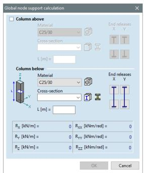
Here, stiffnesses of the support can be automatically calculated if the main parameters are specified for (lower/upper) columns.
