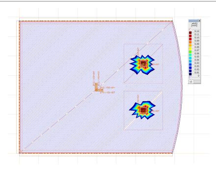
To determine the deflection of the cracked slab you need to run **Nonlinear static analysis** considering load combination **Co.#1 (SLS)**.
