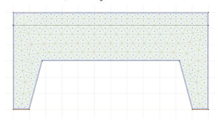
With this final step, the finite element definition of the wall structure has been completed. In the following, we proceed the analysis with this model (*Geometry definition using domains*).
