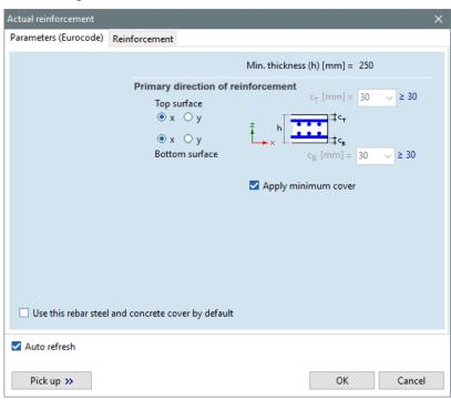
Set **x** direction for **Primary direction of reinforcement** on top and bottom surface on **Parameters** tab and check the **Apply minimum cover** checkbox.
