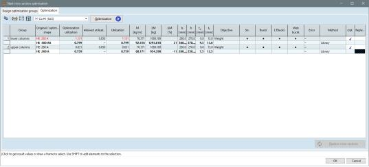
Considering the specified parameters for optimization, the software suggests to apply shape **HE 260 A** for upper columns, and **HE 400 AA** for lower columns.
