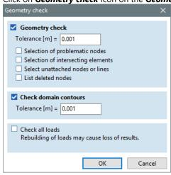
In the window, the maximum **Tolerance** (distance) for checking points can be set. Check the **Select un-attached nodes or lines** checkbox and start the analysis with pressing **OK** button.
