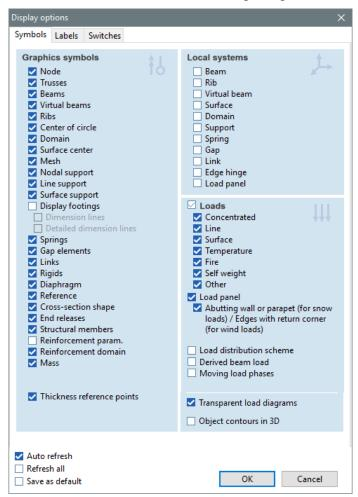
Check Surface checkbox in the Local Systems panel group. Accept the change with OK.
