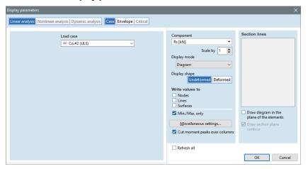
In this window select *Write values to Nodes* function and close with *OK* to see the results:
