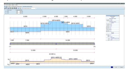
The software generates the actual reinforcement followings the shape of the internal forces by increasing or decreasing the number of rebars.
