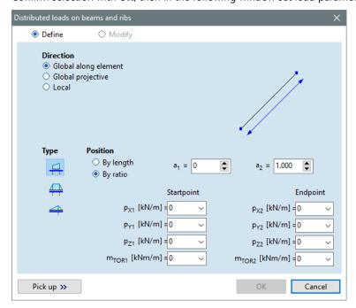
Set  $p_{Z1}$  and  $p_{Z2}$  to -25, then finish with OK, then the load is indicated on the beam elements in cyan:
