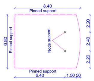
The thickness of the slab is 200 mm, concrete strength is C25/30, the rebar is B500A type. Use Eurocode 2 for design.
