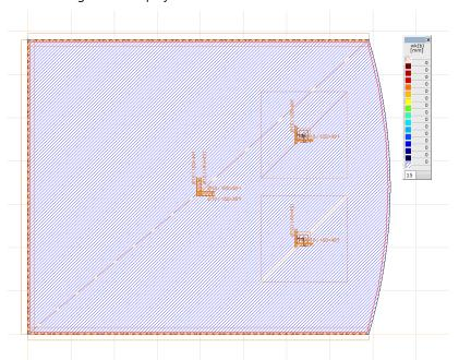
Domain is hatched in blue which means that there are no cracks at bottom surface of domain applying the selected load combination.
