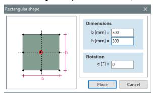
Set **b** and **h** sizes to **300** mm, and click on **Place** button. Click anywhere in the window to place the new cross-section.
