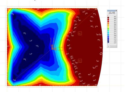
The specified actual reinforcement in local x direction is safe in **Co.#2 (ULS)** load combination because any negative value cannot be seen in the figure.
