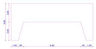
The wall thickness is 200 mm, assume material C25/30 for concrete and B500A for the reinforcement. Analyse the structure according to the Eurocode 2 standard.
