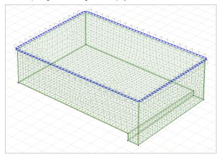
Green points at the centre of surface elements represent *Centre point*s of the shells. Moving the mouse over a centre point, a hint appears after a while showing properties of the finite element.
