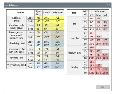
Select type **CST** (**Homogenous, coarse and medium sand,** in **dry or damp** column and **Solid** row), then parameters of the selected soil are shown in bottom left corner:
