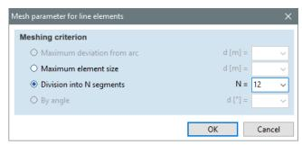
After select the beam element on the right side and divide it into **10** parts with the same method above.
