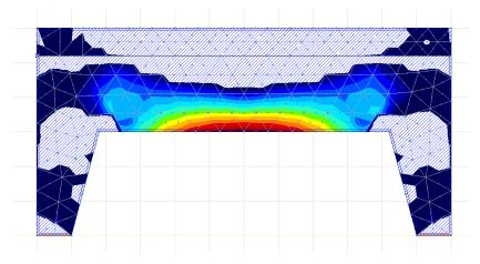
The required specific reinforcement in the x direction is the sum of axt and axb values.
