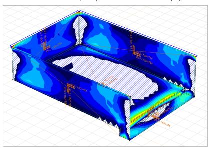
The thick brown lines and their titles indicates the given actual reinforcement. If only one direction of reinforcement is visible on the screen, then open **Display options**. On **Label** tab switch off **According to the displayed result component** function.
