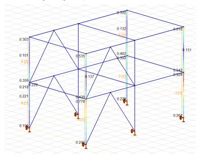
In the figure can be seen, that the maximum utilization of the critical member in the right corner is **0,928** (92,8%) after modification. This result is greater than the value that was set for optimization. This increase is due to the change in internal forces.
