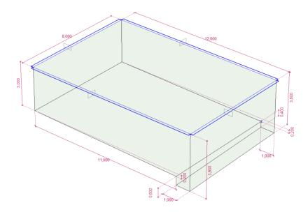
The thickness of the walls and the bottom slab is 250 mmm, the cross section of the ribs on the upper edges is 300x600 mm. The reservoir is made of concrete C25/30, the type of rebar is B500B. Use Eurocode 2 for design.
