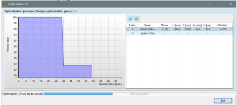
When the optimization process is complete, as a result the suggested cross-section is displayed under the row of the current cross-section:
