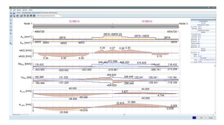
When determining the distribution of longitudinal reinforcement, the given parameters of rebars and the line meshing (see before) are considered.
