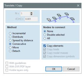
Select **Consecutive** and **None** checkbox under **Nodes to connect** title. Click on bottom node of one of the column, then on the top of it, finally press **Esc** to close command.
