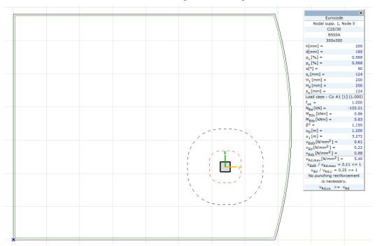
According to the check, **No punching reinforcement** is needed.
