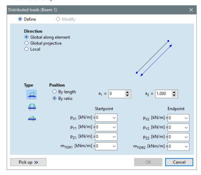
Uniformly distributed load will be defined on the beam relative to the global system. Type in -17.5 into fields  $p_{Z1}$  and  $p_{Z2}$  then confirm with **OK**. The negative value means that the load acts downward, in negative direction.
