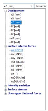
The nx diagram shows the membrane force in local x direction.
