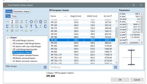
Close window with **OK**, then the selected cross-section is now displayed on the panel:
