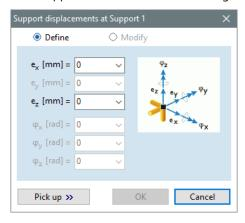
Type in value **20** in field  $e_z$ . During data input always observe signs and directions. If necessary, switch on the local coordinate system of the support (Display Options icon/ Symbols tab/ Local systems group/**Support** checkbox). The color coordinate system show the x, y and z directions (x - red, y - yellow and z - green).
