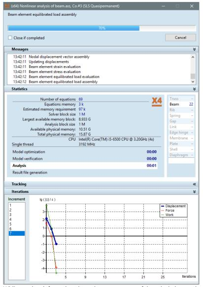
While running, information about the current steps of the calculation can be seen in the **Messages** list. In the **Iterations** window, the actual convergence of the calculation is presented during each increment.
