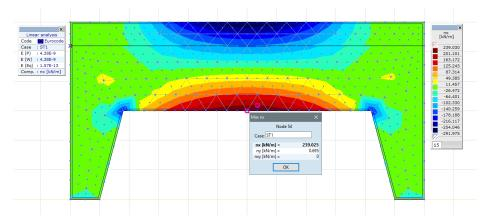
The **Color legend** shows boundary values of each colour. Adjust number of colors and boundary values by dragging up or down the bottom edge of the palette.
