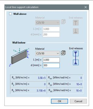
Confirm settings with **OK** and the calculated values are displayed at the components in **Line support window**. Click on **OK** to close the window and the following will be displayed in the main window:
