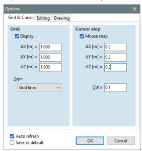
With these settings, the mouse cursor moves in **0.2** *m* steps (geometric imperfection or editing error can be avoided while drawing the model).
