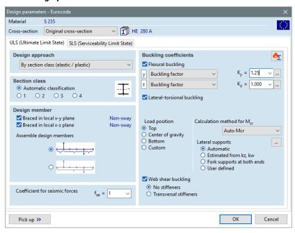
Set  $K_y$  to 1,25-re, and select **Auto Mcr** method to calculate  $M_{cr}$ , and close window with OK.
