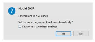
Check the **Save model with these settings** checkbox and degree of freedom settings will be saved. Accept **Membrane in X-Z plane** setting and close with **Yes** button.
