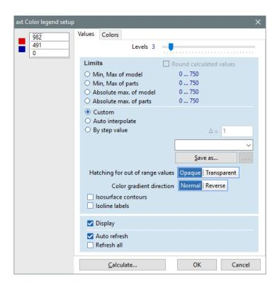
Close settings with **OK**, then the program separates areas by colors where the specified reinforcement spacing is still sufficient.
