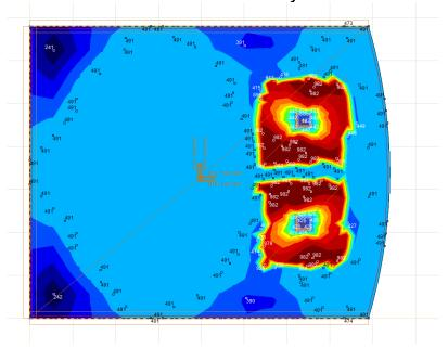
Now, the results of **yt – ayt** component are positive, so the actual (defined) reinforcement is sufficient for all reinforcement layers.
