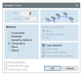
Close window with **OK** and define translation vector by clicking on lower and after on upper nodal support. Performing these steps, we have copied the actual **domain reinforcement**, the following will be displayed:
