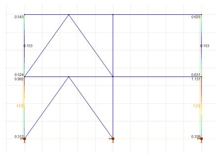
The lower right column is not safe for the load combination, because the maximum utilization (1.131) exceeds value 1. The design error will be corrected by using **Optimization** function.
