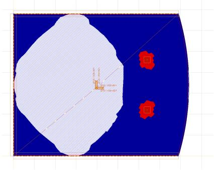
The thick brown lines and the titles indicates the given actual reinforcement. If only one direction of reinforcement is visible on the screen, then open **Display options**. On **Label** tab switch off **According to**
