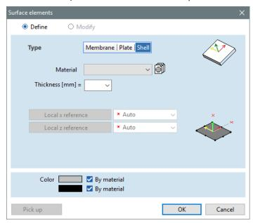
Set Type of the element to Membrane (plane stress).
