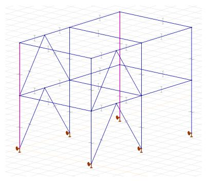
then apply **6** kN/m line load in **x** direction ( $p_{X1}$  and  $p_{X2}$ ). The same way, apply **12** kN/m to the central column in **x** direction.
