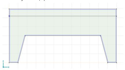
The blue line on the inner contour of the domain indicates the type of the domain (in our case it is membrane). Moving the cursor over it shows a hint window with the properties of the domain:
