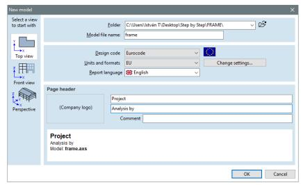
Starting workplane also can be set on the left in this window. Change workplane to **X-Y Top view**. This setting can also be done using **Choosing view** icon on the editing interface.
