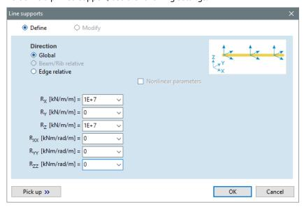
With this final step, the finite element definition of the wall structure has been completed.
