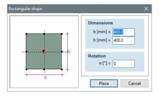
Finishing the data input, press **Place** button to place the cross-section in the editor window. Click anywhere in the window. We get the next result:
